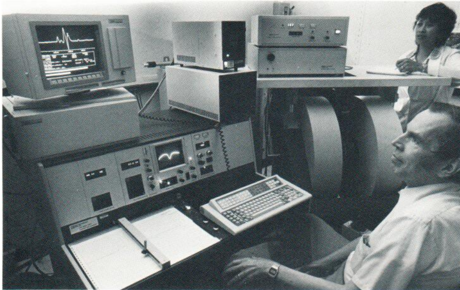
Dr. John Seidel studying the flexibility of the myosin molecule by electron spin resonance.
