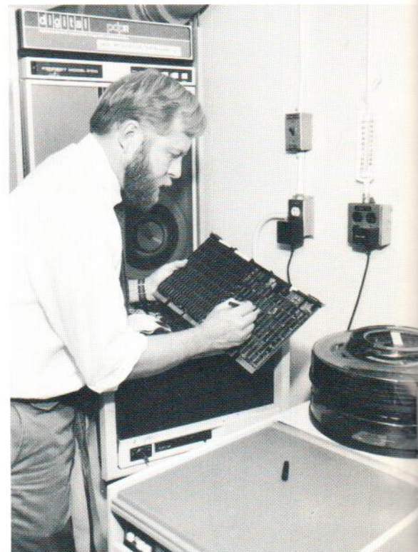
Dr. Walter Stafford installing a memory expansion board in the Digital computer facility which preceded BBRI's impressive new DEC system. The new system was made possible by a generous equipment grant from Digital Equipment Corporation.
