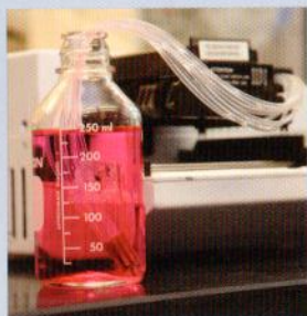
BBRI's new liquid dispenser can transfer micro-liter volumes of fluids with high accuracy in fewer than 15 seconds.
