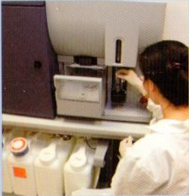
Special sensors monitor how a cell scatters light in order to determine properties such as size and cell complexity.
