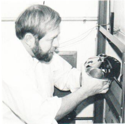
Walter Stafford loading an analytical rotor containing a sample of muscle protein into the ultracentrifuge.
